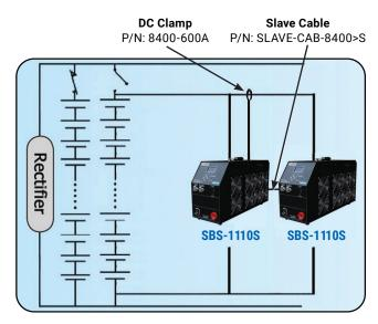
With the optional P/N 8400-600A DC clamp the user can parallel additional load banks of the same voltage range to increase discharge current.
