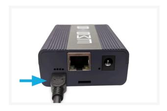
Power the Mini Gateway by connecting the mini USB to the mini Gateway
