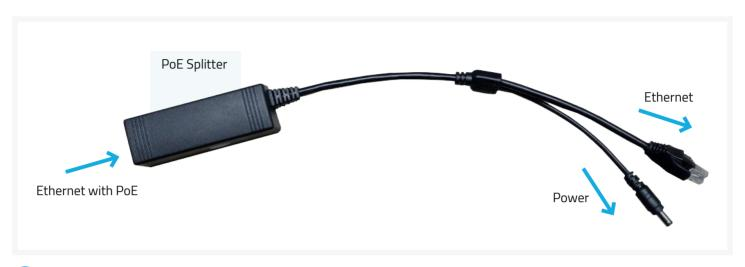
Connect the PoE enabled Ethernet cable into the female LAN port of the PoE splitter.
