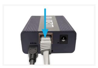
Connect the Ethernet cable into the Mini Gateway's Ethernet port
