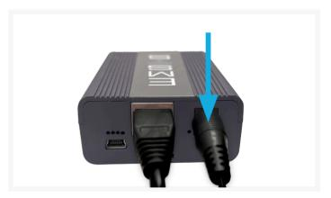
Connect the male LAN connector and the power connector to the Mini Gateway's Ethernet and power connector.
