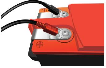
Plug the **red** connector onto the tab of the positive post
