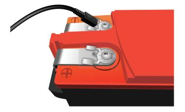
Plug the **black** connector onto the tab of the negative post
