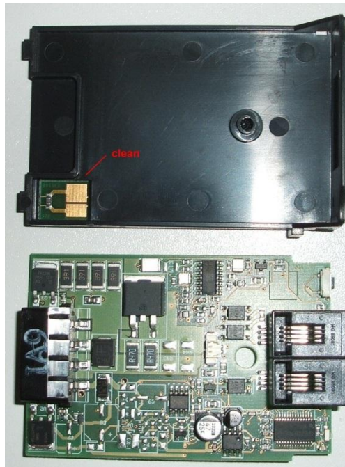
Figure 91: EQUALINK C Module Main Board and Dust Box
