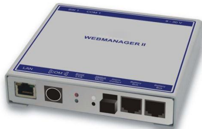
Figure 5: EQUALINK WEBMANAGER II with Integrated EQUALINK CONVERTER
