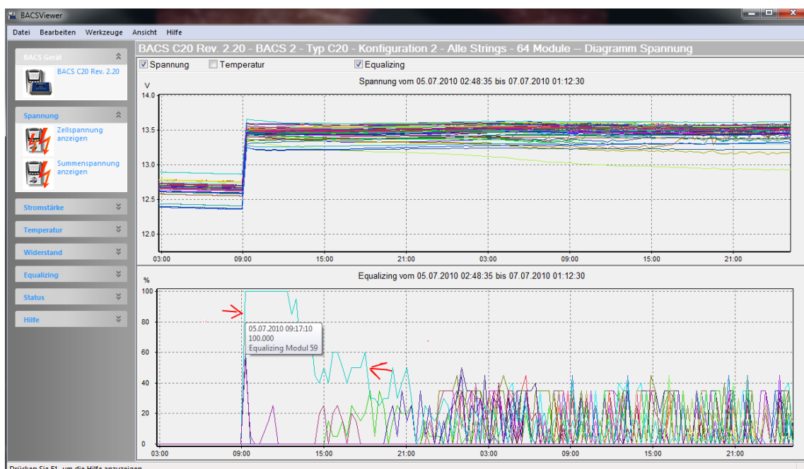
Figure 66: EQUALINK Balancing Chart, showing the effect of Balancing on battery No. 59, avoiding overcharge.
