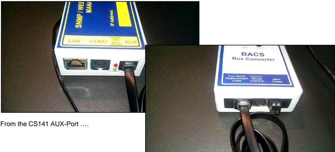
... to the COM 3 port of the EQUALINK-Bus Converter
