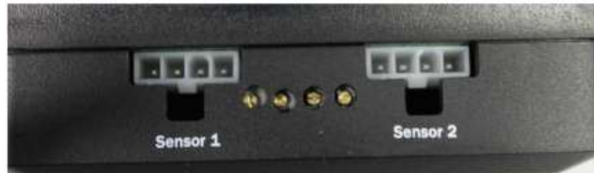
Calibration Potentiometers (Left to right: Warning1, Alarm1, Alarm2, Warning2)
